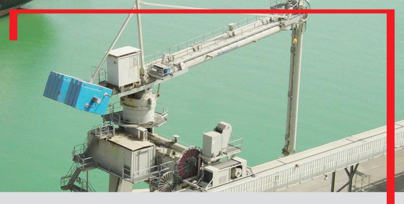
The Movalbe transfer trolley is mounted on the quay conveyor, which has the same length as the ship and runs parallel to the quay edge. The quay conveyor can be of either belt or screw type. It is built in a trough, which is covered by a special rubber belt.
