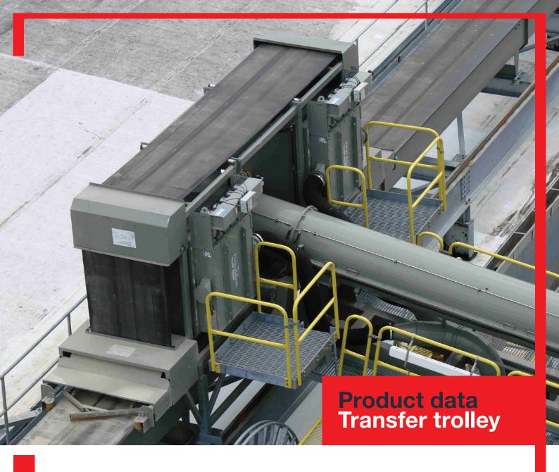
A typical Siwertell continuous screw-type ship unloader travels on rails along the quay. The unloaded material must often be transferred from the travelling unloader to a fixed conveyor on shore. The Movable transfer trolley makes it possible to perform this material transfer without dust and spillage.
