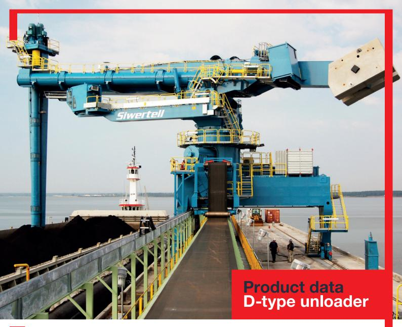
The Siwertell D-type is the heavyduty machine of the continouos Siwertell screw-type ship unloaders. The D-type offers high capacity and ability to unload large vessels. at the point where the offloading gantry conveyor of the unloader is located.
