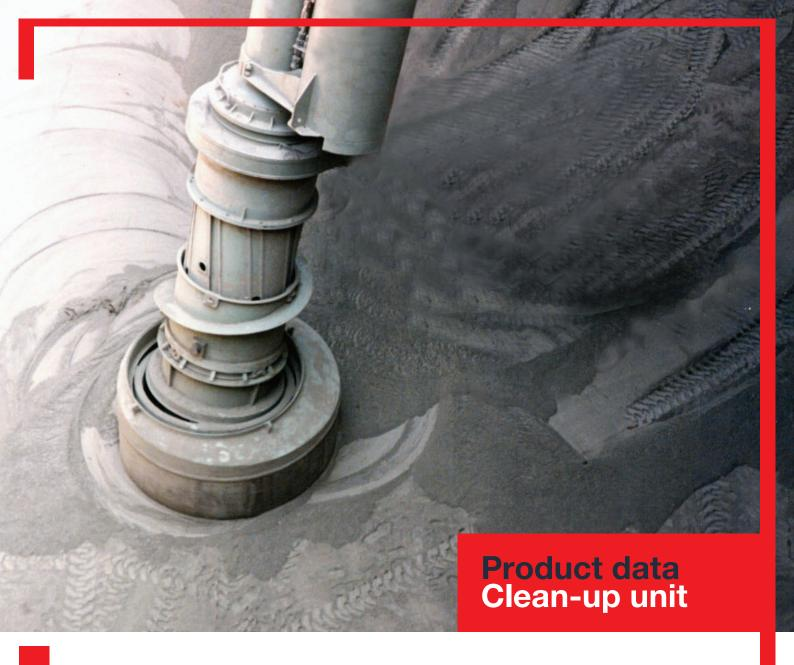
The clean-up unit for Siwertell unloaders can be used during the clean-up phase when unloading free-flowing materials such as cement or granulates. It is shaped like a spiral which, while rotating, collects and pushes the material inwards towards the inlet device and the vertical conveyor in the centre.
