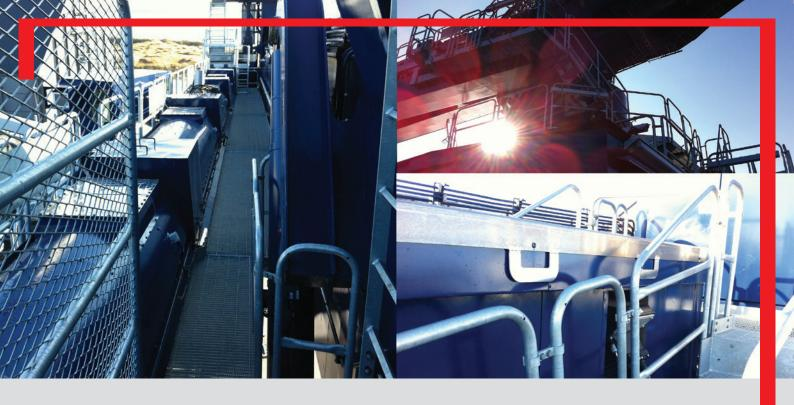
Siwertell design follows applicable international and national safety standards in the country of installation, and are designed specifically for each application. For example, standard off-the-shelf access ways are not easily adopted to a ship unloader without compromising the function. Siwertell therefore uses its own engineering and manufacturing network.
