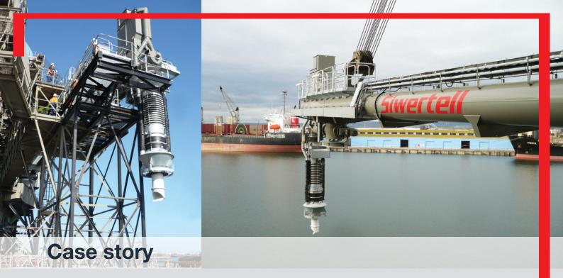
The new conveying system was needed to reduce dust emissions and increase the system's loading capacity, especially for cement.
