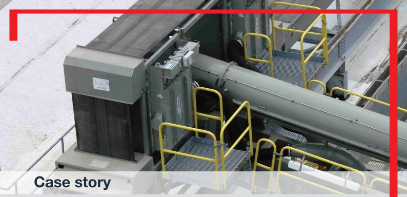
All conveyors, from pick-up in the ship's hold to the storage area are totally enclosed and provide a clean and spillage free operation. This criteria was one of the most important ones for the customer when selecting the Siwertell equipment.
