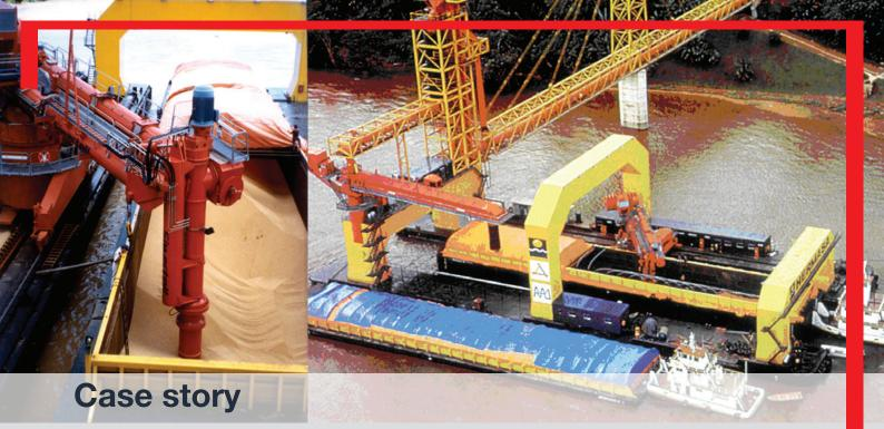
The Siwertell continuous screw-type barge unloader, travelling on rails along the length of a catamaran-type pontoon, plays an important role in a floating grain transhipment terminal installed at Itacoatiara on the Amazon River in Brazil.
