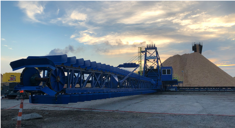
CANTILEVER CHAIN RECLAIMER
