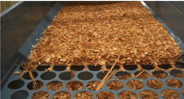
Guide fins in the trough bottom help to orient material so that short wood waste, for example, has a better chance of being chipped properly, improving chip quality. Infeed conveyors can be equipped with a capacity control that reacts to the chipper's motor load.
