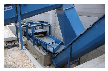
Their totally-enclosed design delivers an environmentally-friendly profile, ensuring that dust emissions and spillage are eliminated when handling all materials. Our screw conveyors also have low energy consumption demands, further adding to their environmental credentials.
