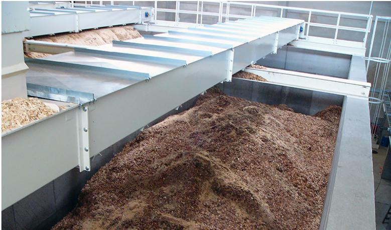
Bruks' drag-chain conveyors employ a heavy-duty chain and paddle transport arrangement that effectively traps and drags material between the paddles along the length of the conveyor to its end destination.
