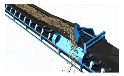
Belt-type conveyors can easily be equipped with additional features to tailor them for an operation. These include optional trippers or belt ploughs for distributing and stacking materials. They can also have ridged, otherwise known as cleated, belts for high conveyor inclination and be fitted with covers for dust and moisture control. Optional covers and spillage plates ensure clean, spillage free belt conveying with minimal dust creation.
