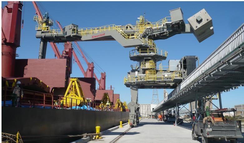
We can find the perfect match and offer the market's highest through-ship efficiencies. Our large-scale ship unloaders have capacities up to 3,000t/h and can be installed as a fixed unit, or rail-mounted for traveling along the quayside. For smaller scale operations that require degrees of mobility, we offer road-mobile units and port-mobile units.
