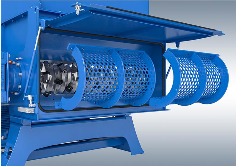
Image: The screen basket and inserts, which can be rotated, are designed in two parts and held securely in position with clamps. Screen perforations are dimensioned according to the required final product.
