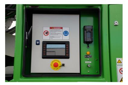
Unloaders with these advanced PLC systems have almost unlimited trouble-shooting potential, both on site and remotely, including the ability to conduct self-diagnostic system runs and software upgrades directly from Bruks Siwertell. The fieldbus system also allows for a significant reduction in cabling, in comparison to older models, throughout the equipment.
