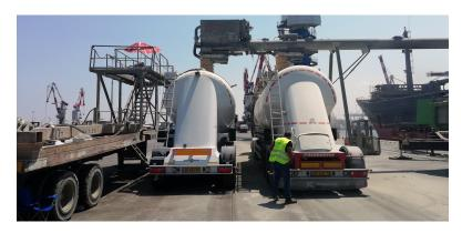
The double-bellows system makes it possible to load at two points alternately using internal slide gates, ensuring that unloading can continue during truck or wagon changeovers. This feature can be automatically-controlled via the PLC or manually from the wireless control box.
