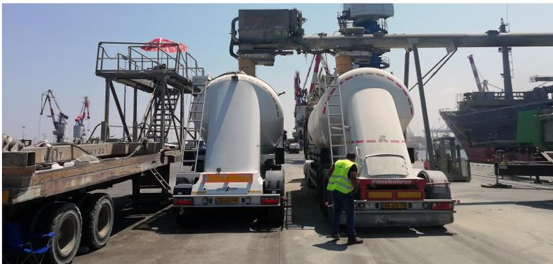
The double-bellows system makes it possible to load at two points alternately using internal slide gates, ensuring that unloading can continue during truck or wagon changeovers. This feature can be automatically-controlled via the PLC or manually from the wireless control box.
