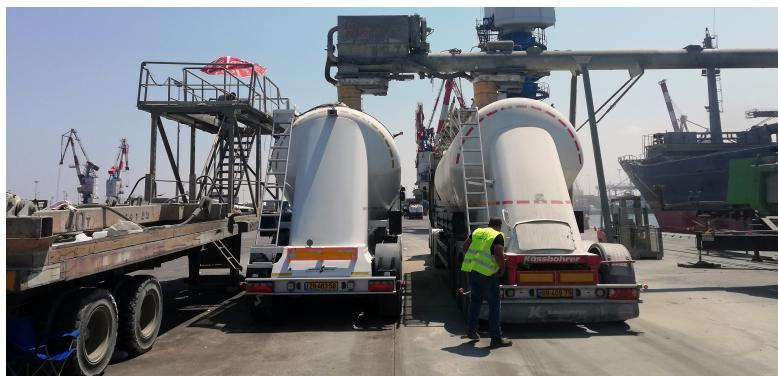
The double-bellow system makes it possible to load at two points alternately using internal slide gates, ensuring that unloading can continue during truck or wagon changeovers. This feature can be automatically-controlled via the PLC or manually from the wireless control box.
