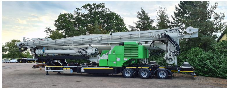
It takes less than an hour to complete the unfolding operation once the unloader arrives on site. Packing away at the end of unloading is equally quick, and these tasks can be carried out by a single operative.
