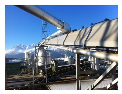
Integral to Granule 777's operation is a new air-supported conveyor system with a rated capacity of 800t/h for carrying wood pellets. It comprises a 100m-long Bruks The Belt Conveyor and a 250m-long Tubulator. The Belt Conveyor carries material from the facility's two pellet storage domes, before transferring it to the Tubulator system which feeds it to the dock where the pellets are loaded onto bulk carriers bound for Europe.
