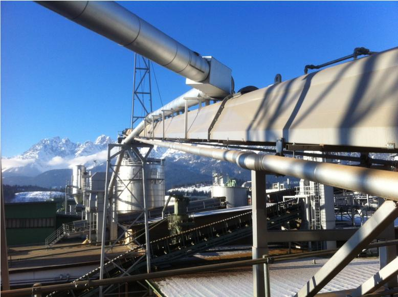
Integral to Granule 777's operation is a new air-supported conveyor system with a rated capacity of 800t/h for carrying wood pellets. It comprises a 100m-long Bruks The Belt Conveyor and a 250m-long Tubulator. The Belt Conveyor carries material from the facility's two pellet storage domes, before transferring it to the Tubulator system which feeds it to the dock where the pellets are loaded onto bulk carriers bound for Europe.
