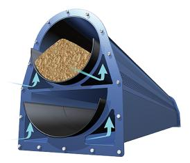
The Tubulator comes in two basic forms: one is totally enclosed on the transport and return sides using an air carry return (ACR). In this version the return belt is supported on a cushion of air provided by a separate blower. The second alternative design uses rollers with 3m spacing to support the return side belt, or roller carry return (RCR).
