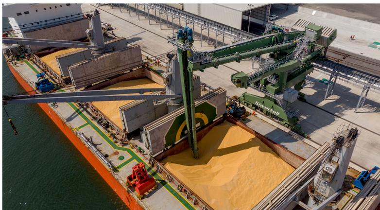
Efficient, clean conveying and grain storage systems and reclaiming technology can be matched to our grain handling ship unloaders and loaders.
