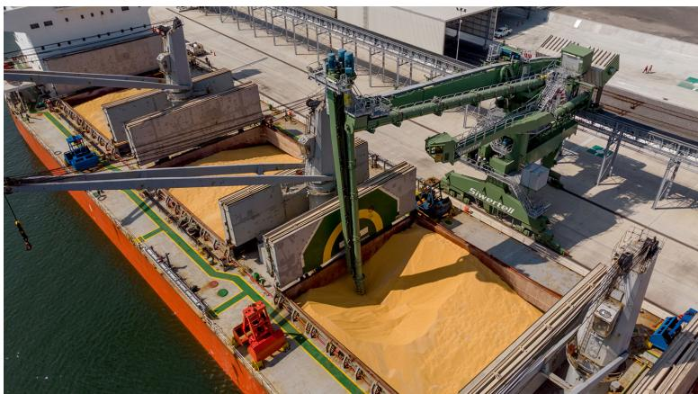
Efficient, clean conveying and grain storage systems and reclaiming technology can be matched to our grain handling ship unloaders and loaders.
