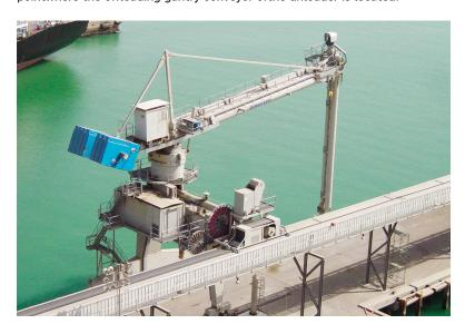
The gantry conveyor of the unloaderis connected to the Movable transfertrolley. The cargo is fed through the Movable transfer trolley on to the quayconveyor. The unloader can travel alongthe quay conveyor and still operate atfull capacity.
