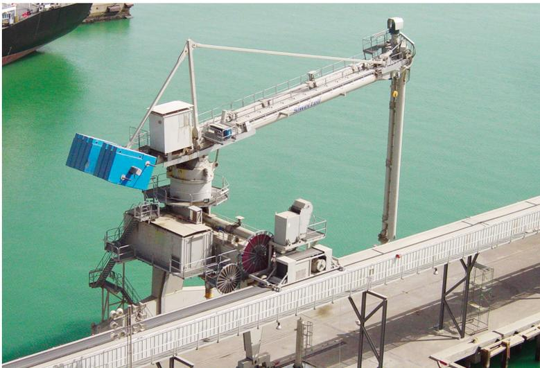
The gantry conveyor of the unloader is connected to the Movable transfer trolley. The cargo is fed through the Movable transfer trolley on to the quay conveyor. The unloader can travel along the quay conveyor and still operate at full capacity.
