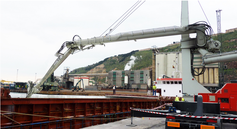
SIWERTELL ROAD-MOBILE UNLOADER - SPAIN
