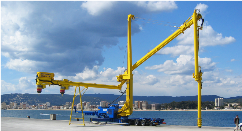
SIWERTELL ROAD-MOBILE UNLOADER - SPAIN
